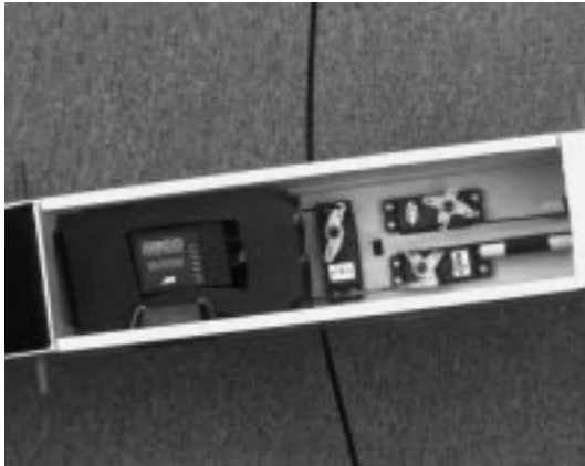
Fuselage Servo, Receiver, Battery Installation
