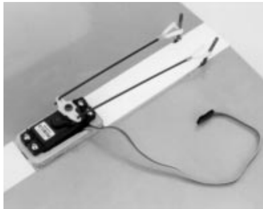
Aileron (Wing) Servo Installation
